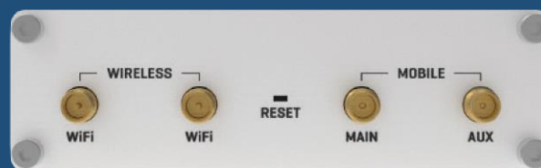
Wi-Fi antenna connectors
